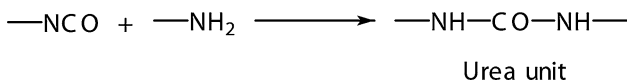
Fig. 10 Reaction between isocyanate and aminic groups with formation of a urea unit
